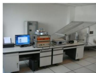
GTEM Cell Radiated Immunity test system
